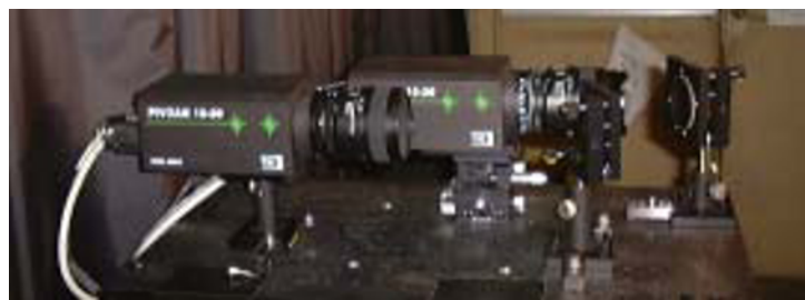
Fig. 2. The photograph of the PIV-PLIF simultaneous image recording system.
